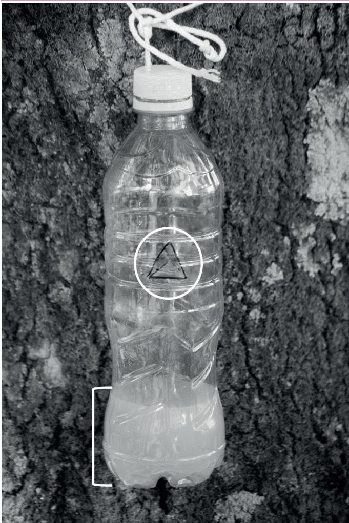
Figure 1. The triangular side opening of 2 cm x 2 cm x 2 cm located 10 cm from the base of the 0.5 L bottle is highlighted in the white circle; the trap filled with 150 mL of artificial juice is highlighted in the white bracket.
